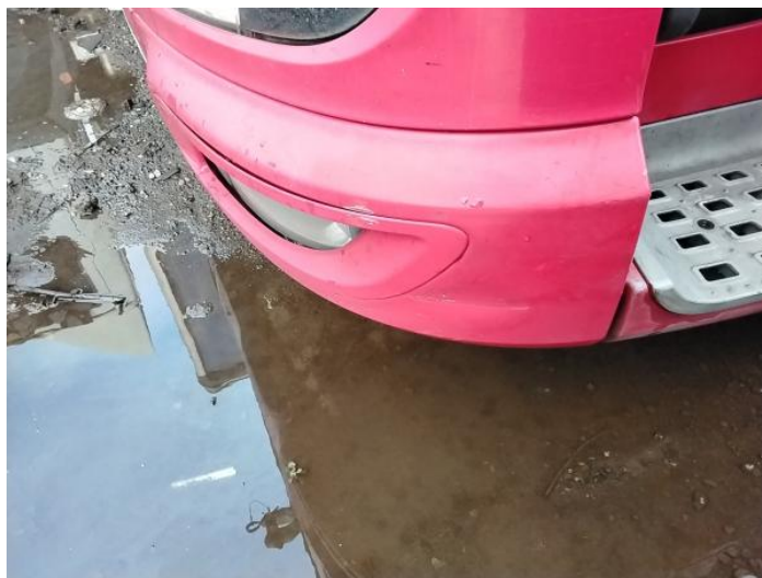
2: Bumper Front Dented Over 30mm
