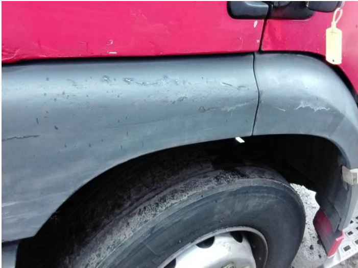
4: Wing osf Poor Previous Repair Rippled Over 30%
